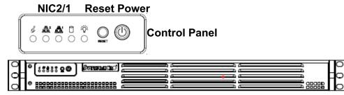
To power off the unit, press and hold the power button for 7 seconds.
