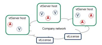
Each vtServer host may run one or more vtAlpha and vtVAX instances. These instances may be either production or 'disaster recovery' instances. Additional host hardware can be provisioned to allow these instances to failover to backup systems, either with manual intervention or automatically. When used with vtLicense servers, the vtAlpha and vtVAX instances will automatically discover their licenses across the network.
