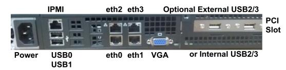
The external USB ports support both vtAlpha and vtVAX license keys. The vtLicense-G3-02/04/06 has two (2) USB ports (shown in closeup below) in the position labeled "PCI slot" in the picture above.
